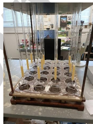
Photo 4. Conditioning of Dowex 50Wx8 resin
