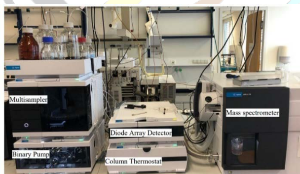
Figure 4. Modules of the LC-MS/MS
