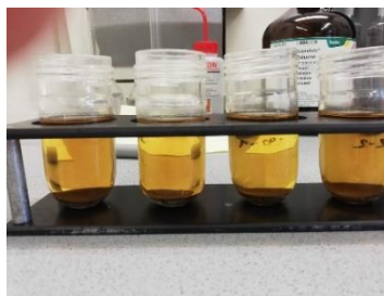
Photo 14. Precipitation of humic acids
