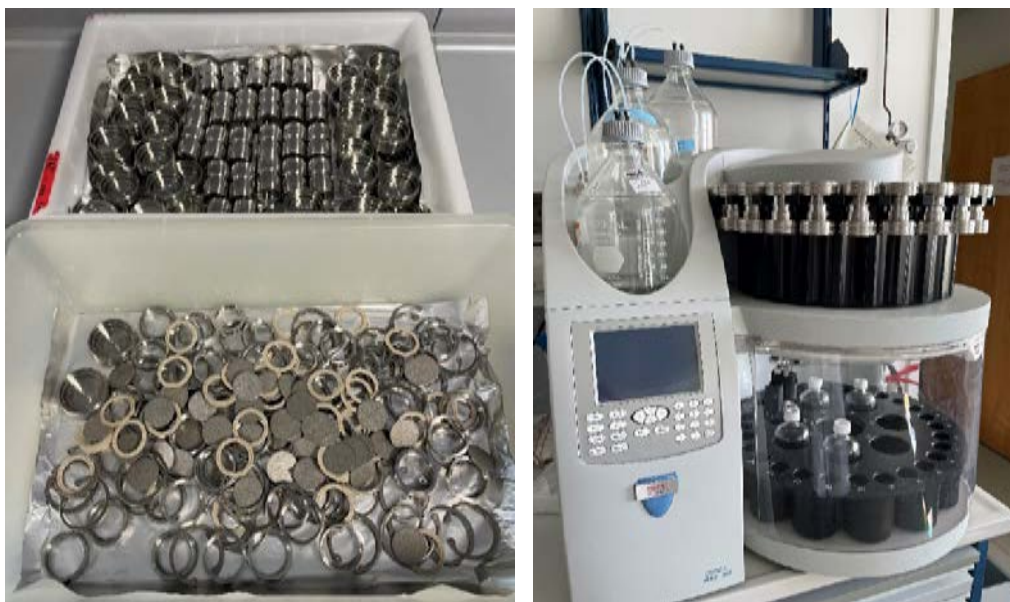
Figure 3. ASE column preparation
