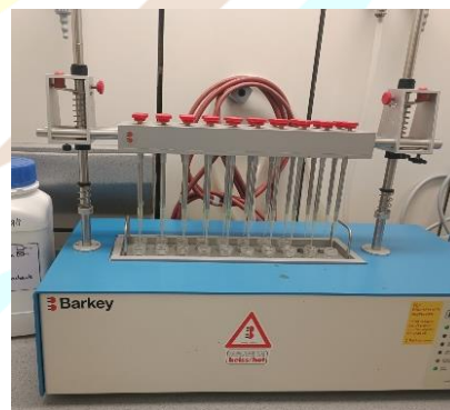
Photo 13. Evaporation in N_2 stream
